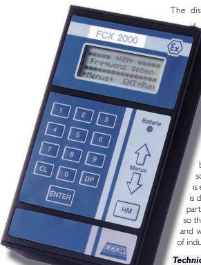
The FCX 2000 offers a simple and quick means of measuring and simulating frequencies, pulses, numbers of revolutions, digital process signals and levels. The operator guidance with the help of a 4-line LCD-display and membrane keyboard allows simple and easy to use adjustment of all operator functions.
